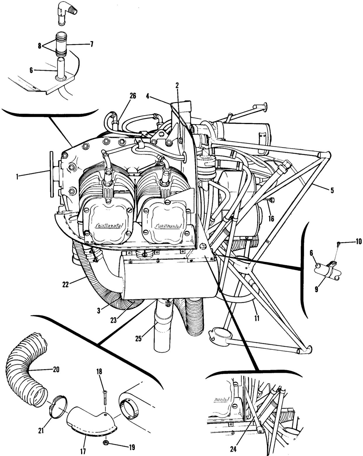
Figure 30. Engine Assembly
