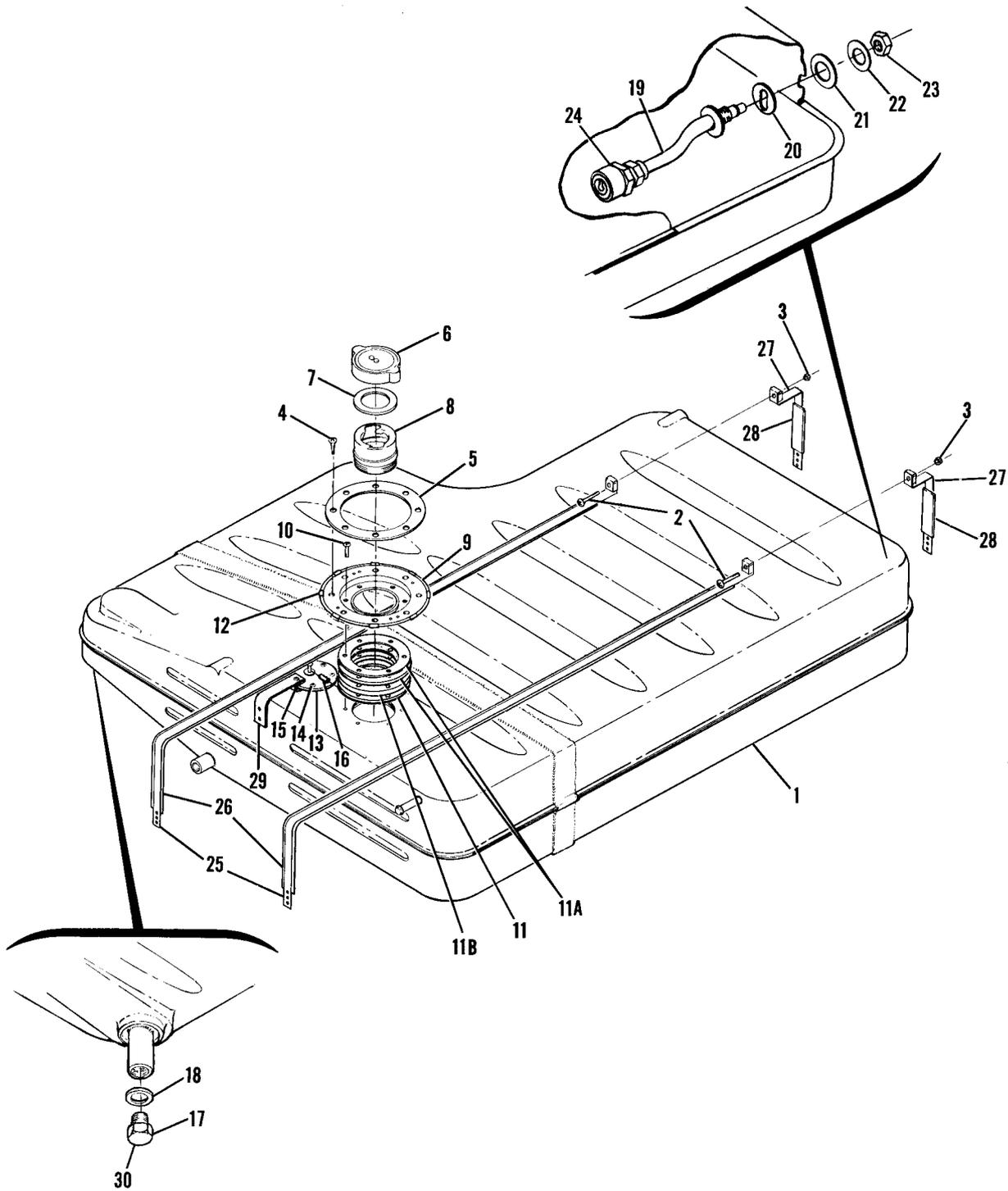
Figure 4A. Patroller Wing Fuel Tank Installation
