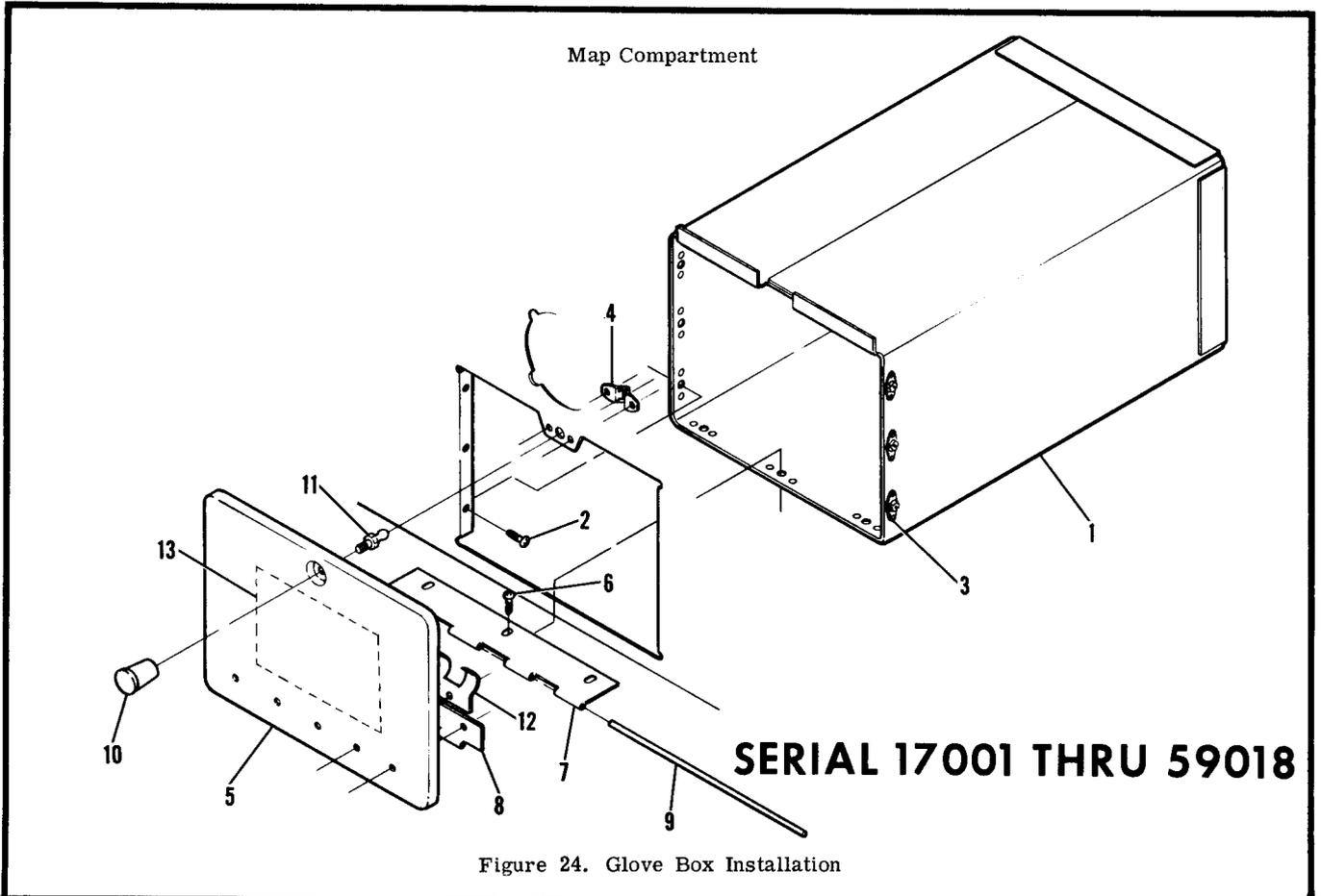
Figure 24. Glove Box Installation
