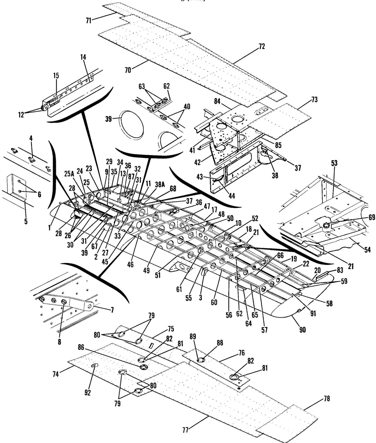
Figure 2A. Patroller Wing Structure Assembly
