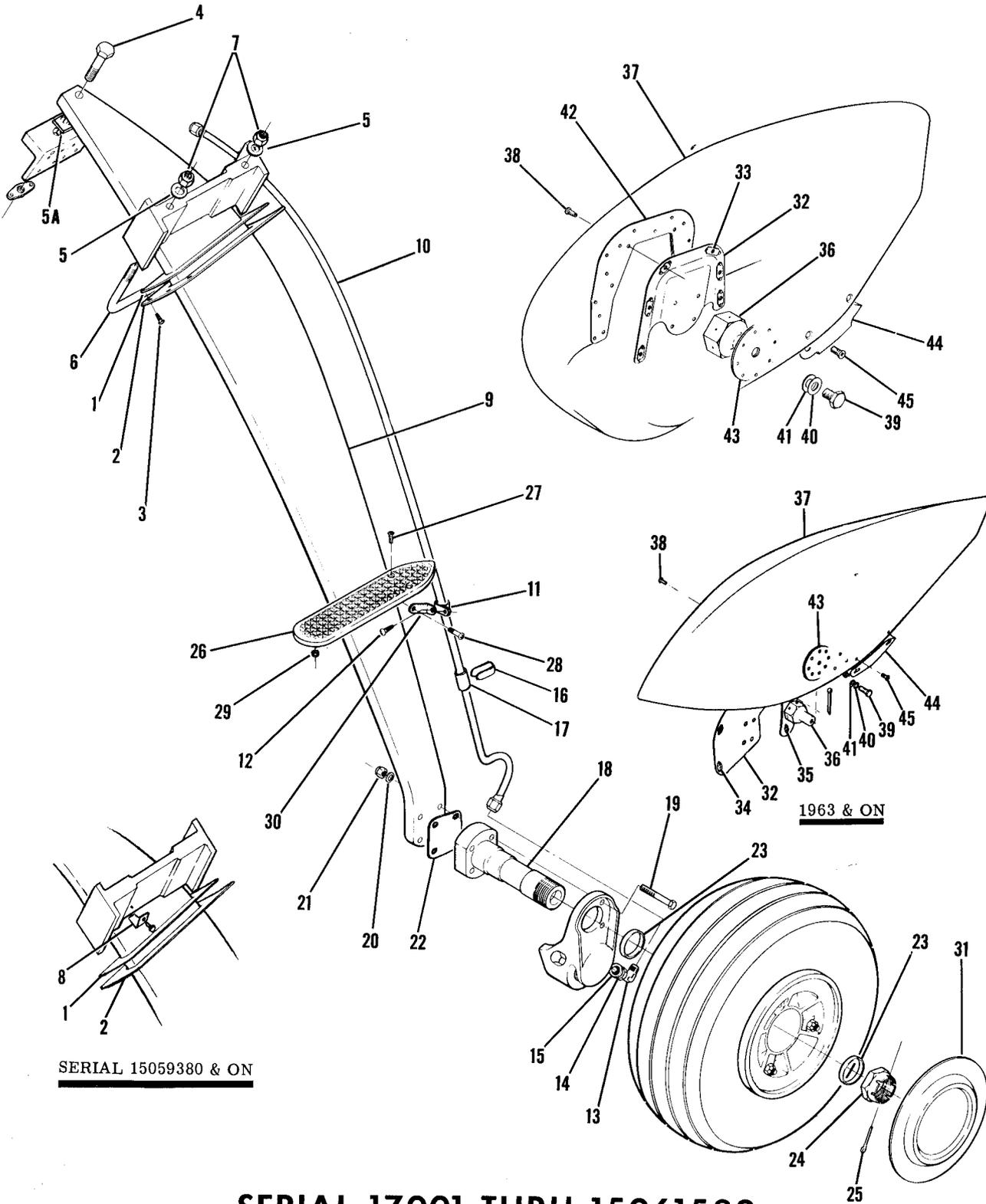
Figure 18. Main Landing Gear Installation
