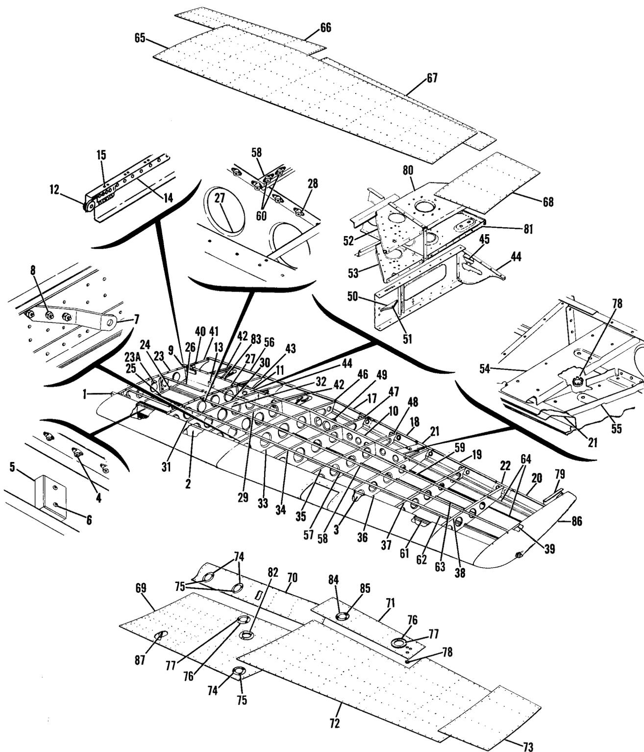
Figure 2. Wing Structure Assembly
