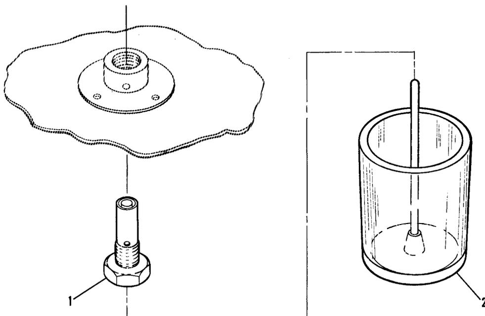
Figure 4B. Fuel Tank Drain Valve Installation
