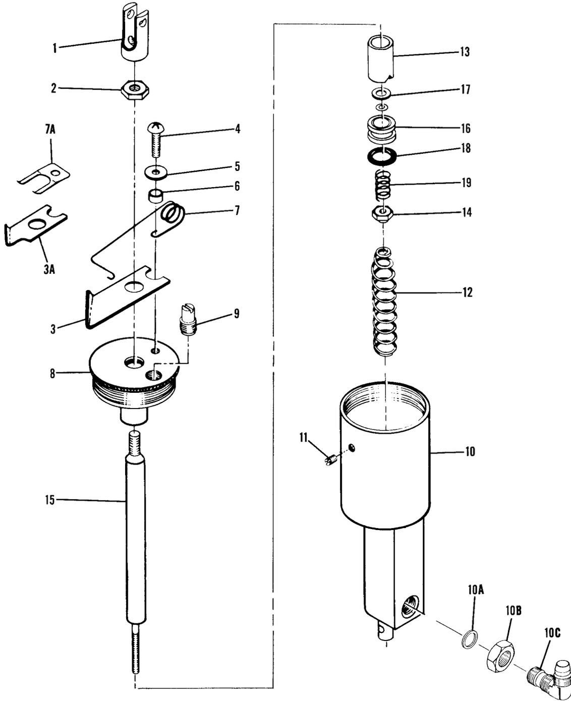
Figure 54. Master Brake Cylinder Assembly
