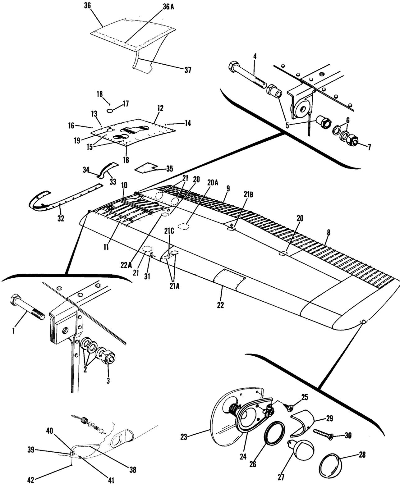
Figure 1C. Wing Assembly Complete
