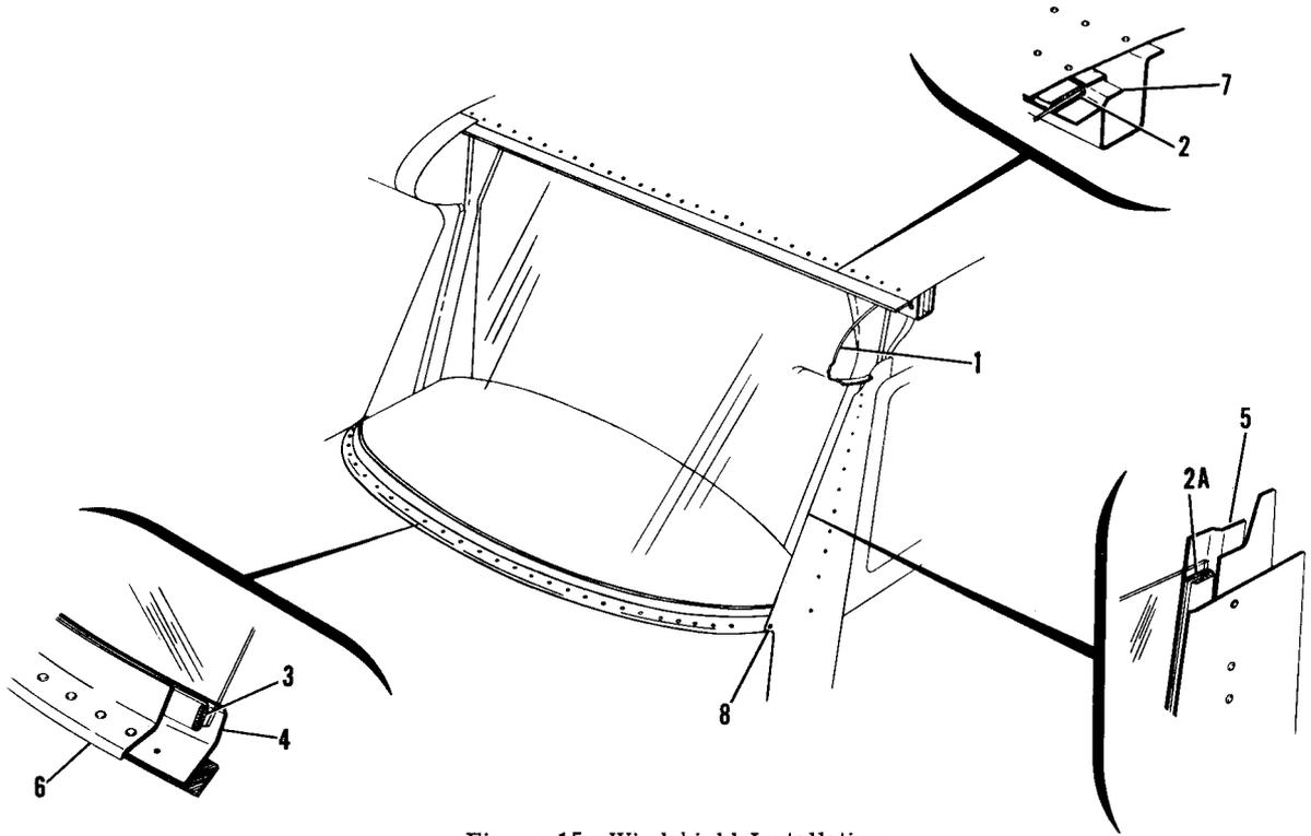
Figure 15. Windshield Installation
