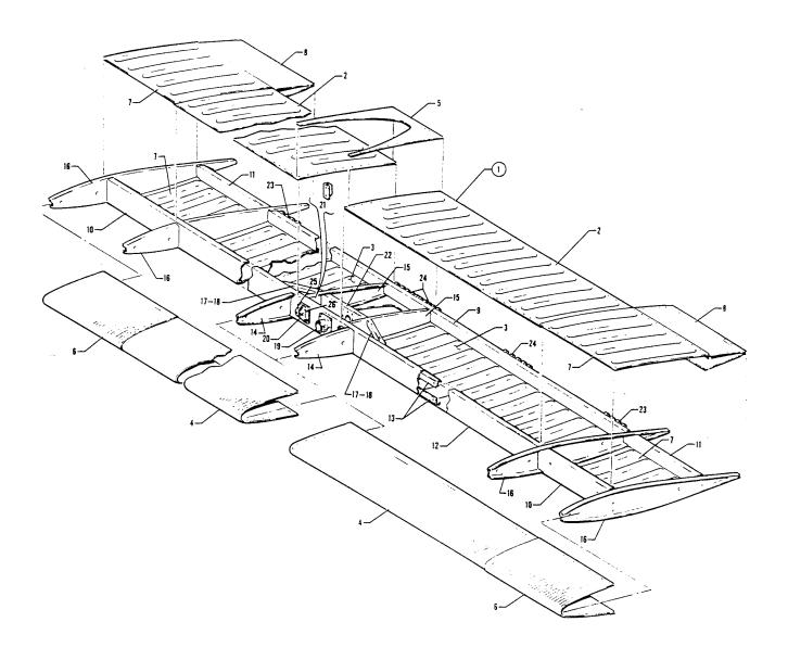
Figure 50D. Stabilator Assembly (PA-28-180 - Serial Nos. 28-7305001 and up) (PA-28-235 - Serial Nos.- 28-7310001 and up) (PA-28R-200 - Serial Nos. 28R-7235001 and up)
