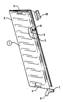
Figure 50B. Rudder Assembly
