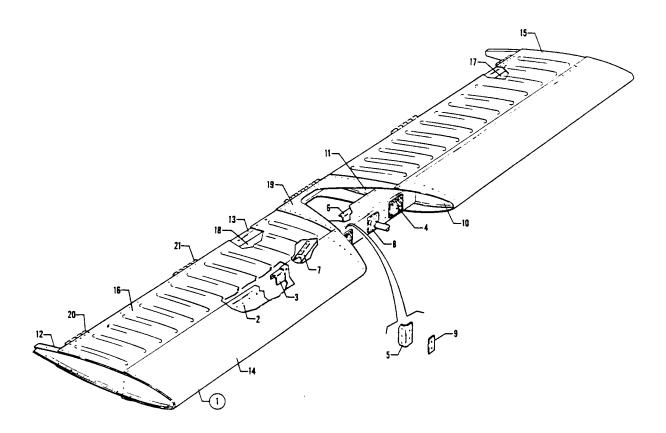
Figure 50C. Stabilator Assembly (See Code "A" on Next Page for Airplane Effectivity)
