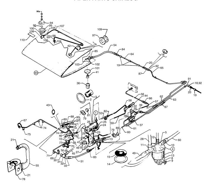
Figure 53. Fuel System Installation (PA-28-150-160-180 - Serial Nos. 28-1761 and up)
