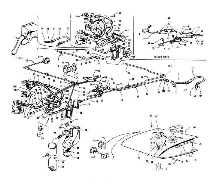
Figure 52. Fuel System Installation (PA-28-150-160-180 - Serial Nos. 28-1 to 28-1760 inclsuive)
