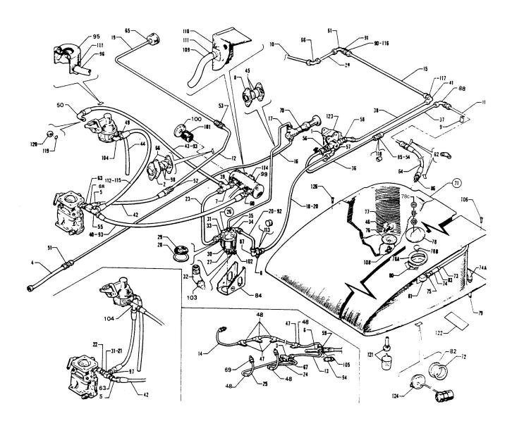
Figure 51. Fuel System Installation
